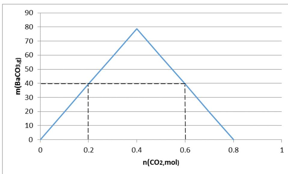
**Pic. 3. Dependence of barium carbonate mass on carbon oxide quantity (IV)**
