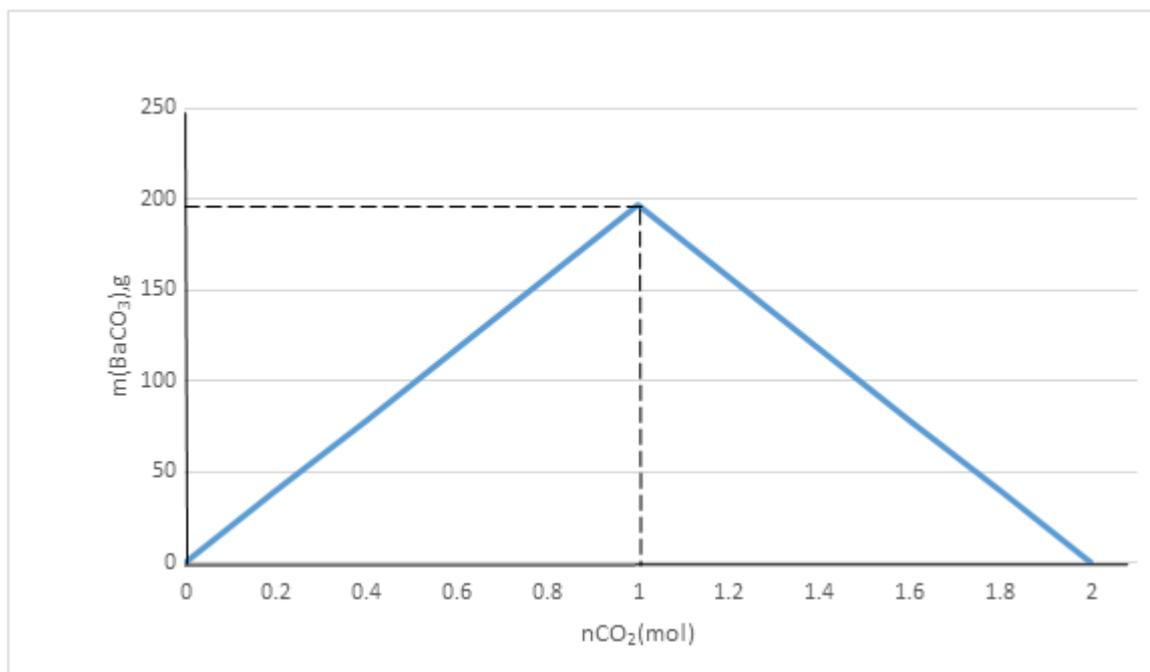
**Pic. 1. Dependence of  $\text{BaCO}_3$  mass on carbon oxide quantity (IV)**
